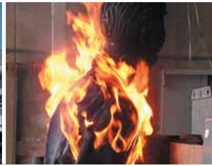
Non-FR 100% cotton after 480v disconnect arc flash.
