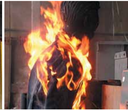
Non-FR 100% cotton after 480v disconnect arc flash.
